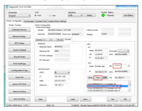
f) IP Choose IP address bar Return to the IP address to search for and enter the corresponding IP address.
