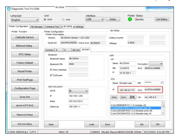
II. Set up the driver to connect to the printer over a wireless network.
