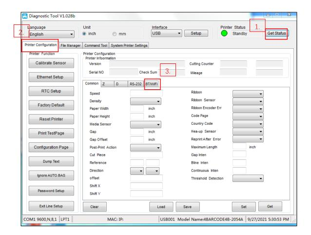
c) Click Get on the bottom right .The Diagnostic Tool will get wireless network parameters.
