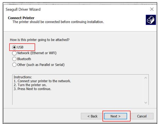
Select the printer according to the actual machine number (which can be viewed on the back label of the machine)
