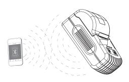
Note: When Bluetooth connects to printer successfully, the buzzer will sound once as a reminder
