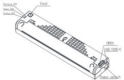
Power LED: High battery show green; Medium battery show red: Low battery show flashing red
